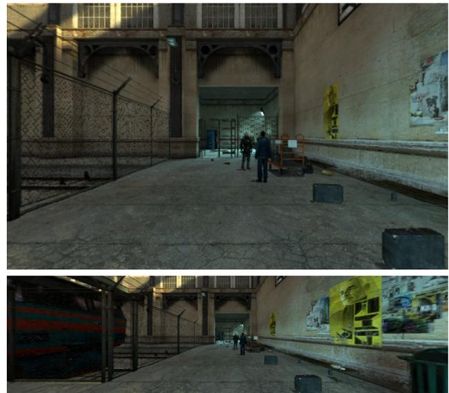
Figure 1. 100 degree (top) and 140 degree (lower) horizontal field of view using a perspective projection.
