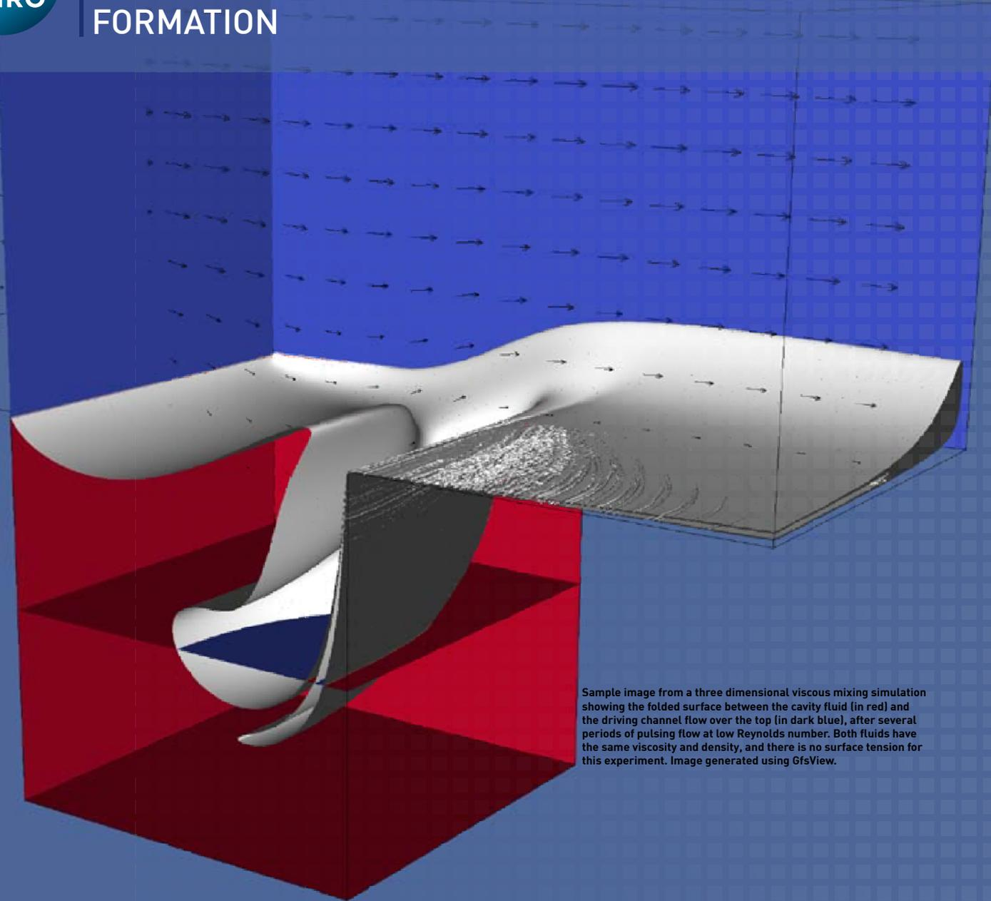
Sample image from a three dimensional viscous mixing simulation showing the folded surface between the cavity fluid (in red) and the driving channel flow over the top (in dark blue), after several periods of pulsing flow at low Reynolds number. Both fluids have the same viscosity and density, and there is no surface tension for this experiment. Image generated using GfsView.
