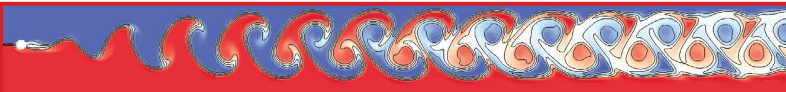
Cylinder benchmark simulating a von Karman street of vortices with diffusing tracer behind a cylinder in moderate-Reynolds number flow. This is a small benchmark used to test Gerris on Epic for small to moderate numbers of processors.
