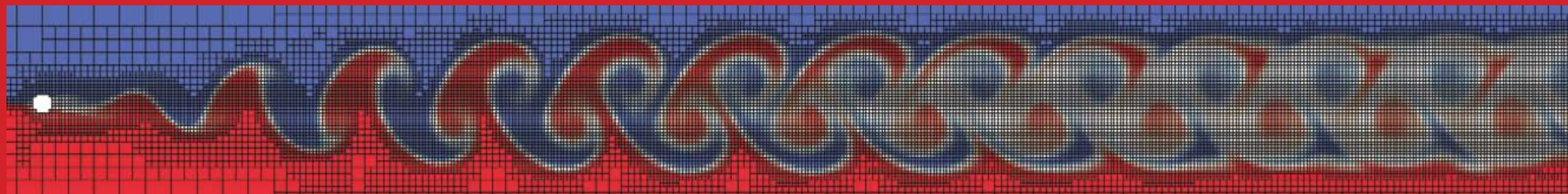
Cylinder benchmark showing dynamically adapted semi-structured grid.
