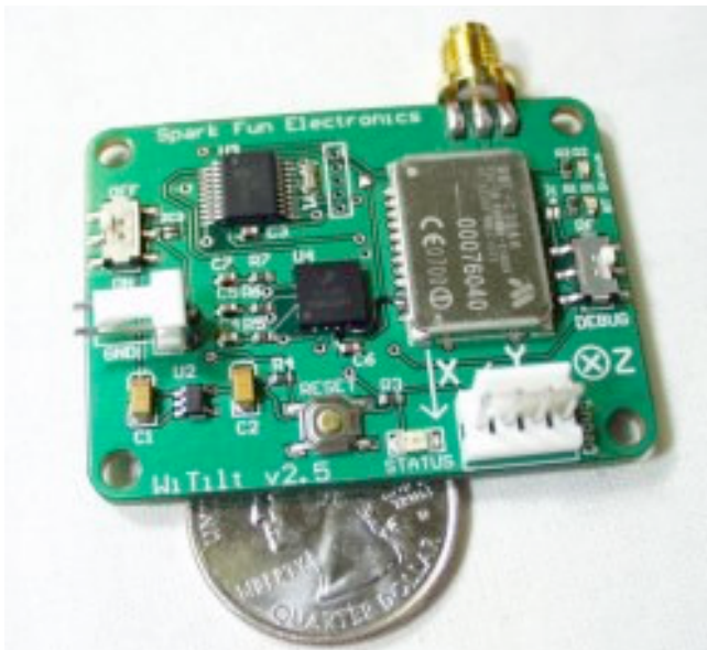
WiTilt v2.5 2.4GHz Wireless 3-axis Tilt Sensor 3/2/2006
