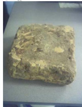
Fig. 2 photograph of an unfired brick taken in Crossley's lab
