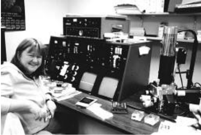
Barbara Plowman at the control panel of a scanning electron microscope. The electron microscope is the cylinder to the far right. Ylem field trip, October 30, 1999. Photo by Robert Ishi.
