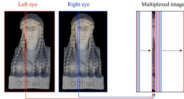
If a barrier strip is placed in front of the multiplexed image at the right distance and spacing then the left eye will only be able to see the left image columns and the right eye will only see the right image columns.
