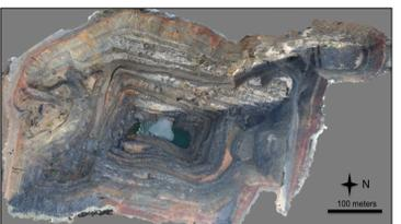
Fig 9. 3D model of Pit in map view. Created using images taken from 50 mm focal length lens.
