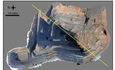
Fig 5. Figure showing impact of shadow on final model.
