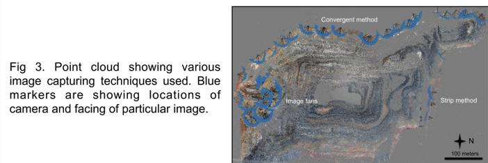
Fig 3. Point cloud showing various image capturing techniques used. Blue markers are showing locations of camera and facing of particular image.
