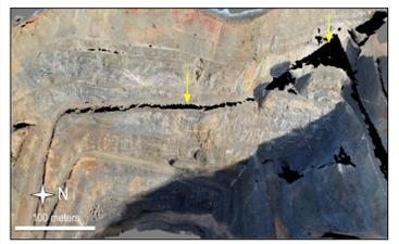
Fig 4. Illustration of occlusion and vertical orientation bias (modified from Sturzenegger et al., 2007).
