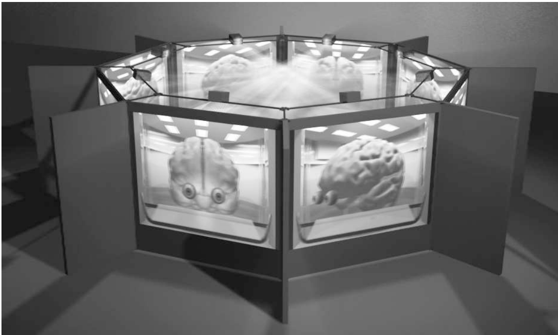
Figure 2: The Virtual Room, an 8-wall, rear-projected stereoscopic system that the audience can walk around in order to see a ‘contained’ version of a dataset. Image by E.Hallein.
