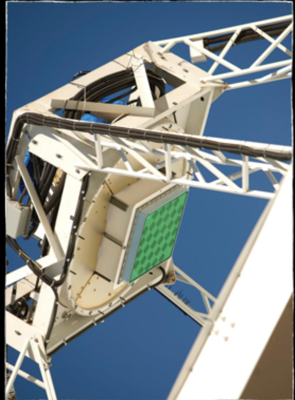
Chequer board sensor array on each dish
