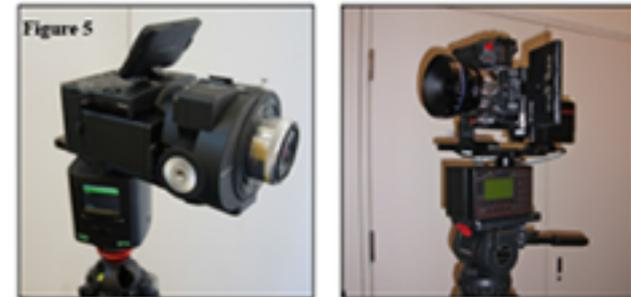
Two technological developments that allow sufficient resolution capture are HD or 4K video cameras, providing 2K or 4K pixel high panoramas, and SLR cameras with fast continuous capture modes (eg: 6 fps of the Canon 5D Mk III) resulting in 5.5K pixel high panoramas. Note that in both cases the camera is typically mounted in portrait mode and the horizontal resolution is dictated by the field of view of the lens.
