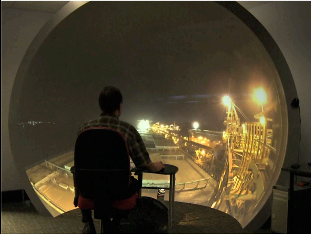
Rio Tinto remote operation ship loader
