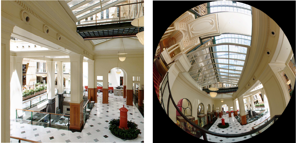
Figure 3. Straight lines in a perspective projection do not appear straight in a fisheye projection.
