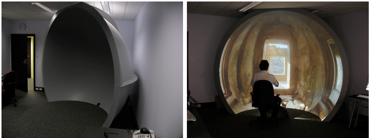
Figure 1. Photographs of the iDome, a 3m diameter hemispherical surface. In the image on the right note the absence of any intrusive projection hardware.
