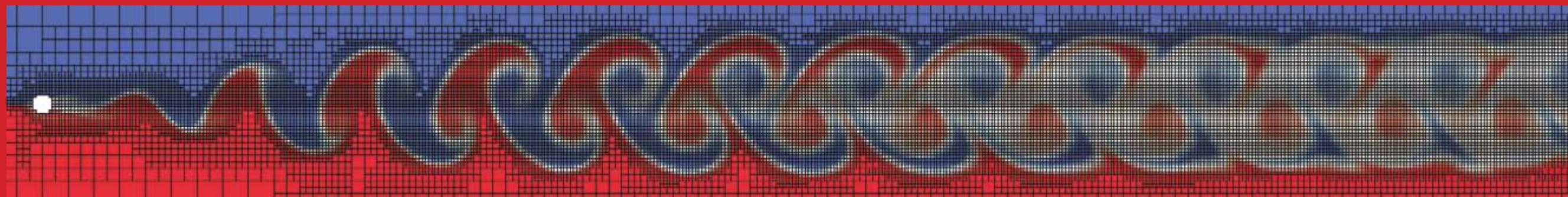
Cylinder benchmark showing dynamically adapted semi-structured grid.
