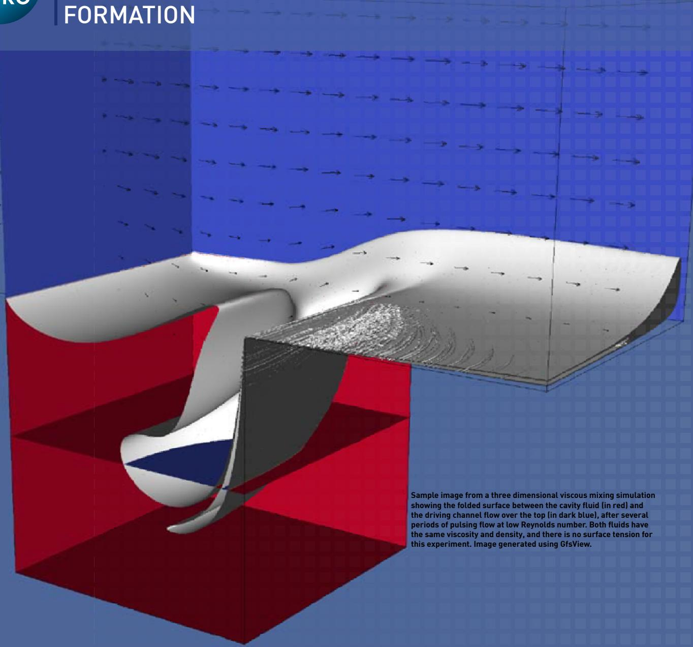
A sequence showing the evolution of mixing between a periodically driven channel flow (blue fluid) and a cavity fluid (red), at moderate Reynolds number ( $Re=246$ , based on the driving flow velocity and cavity width as scales). Image generated using GfsView.
