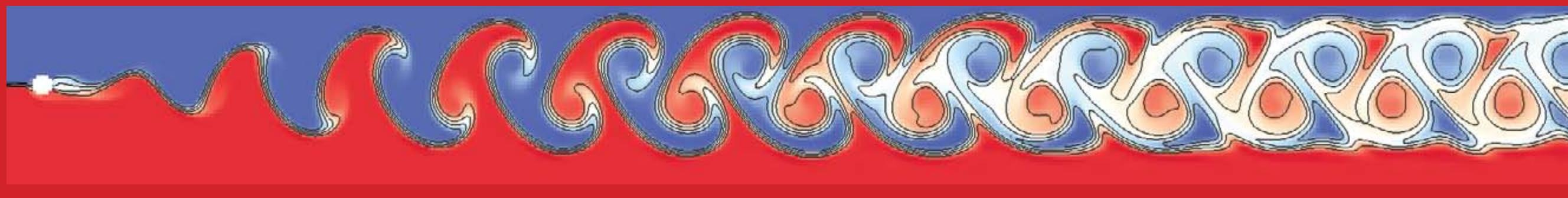
Cylinder benchmark simulating a von Karman street of vortices with diffusing tracer behind a cylinder in moderate-Reynolds number flow. This is a small benchmark used to test Gerris on Epic for small to moderate numbers of processors.
