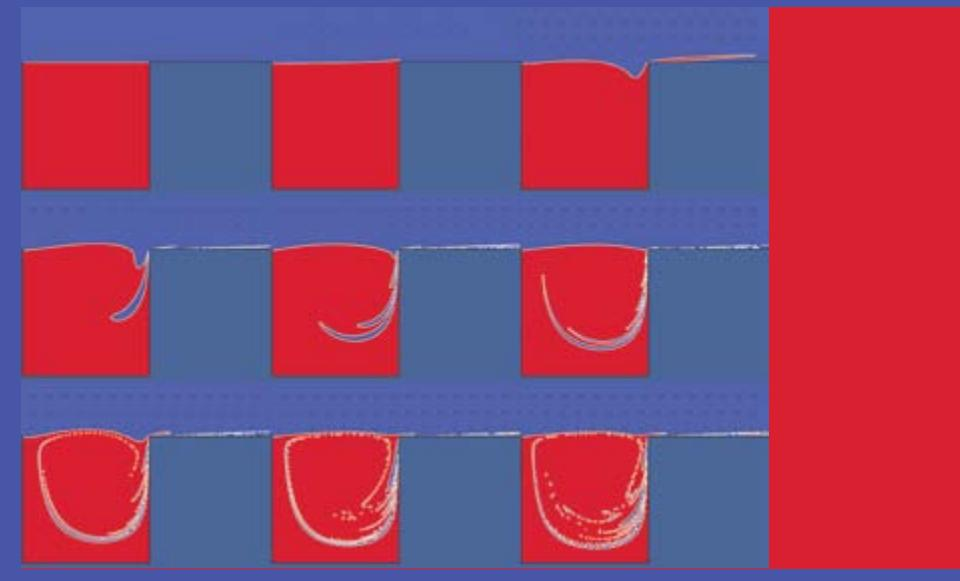
A sequence showing the evolution of the mixture in the cavity under the same conditions as Figure 1, except that the cavity fluid is now denser and less viscous than the overlying driving flow. Image generated using GfsView.
