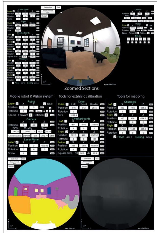
**Figure 1.** Several modes are supported by the simulator. The image above shows ordinary mode. The image below shows semantic labeling mode and depth mode. The middle image shows zoomed sections of the main screen.
