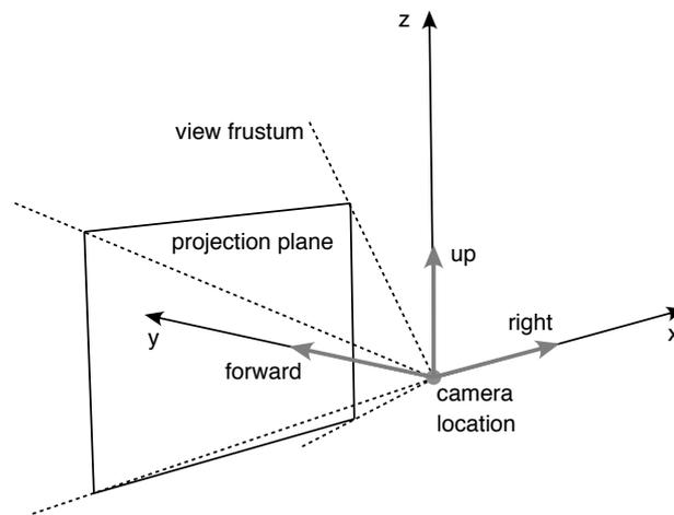
To create a particular perspective view one rotates this initial camera direction and orientation about any axis, or combination of axes. A roll in the chosen coordinate system is a rotation about the y axis (forward), panning is a rotation about the z axis (up) and tilting is a rotation about the x axis (right). To create the 6 faces of the cube map the initial camera view direction is rotated as shown, the horizontal and vertical field of view set to 90 degrees.
