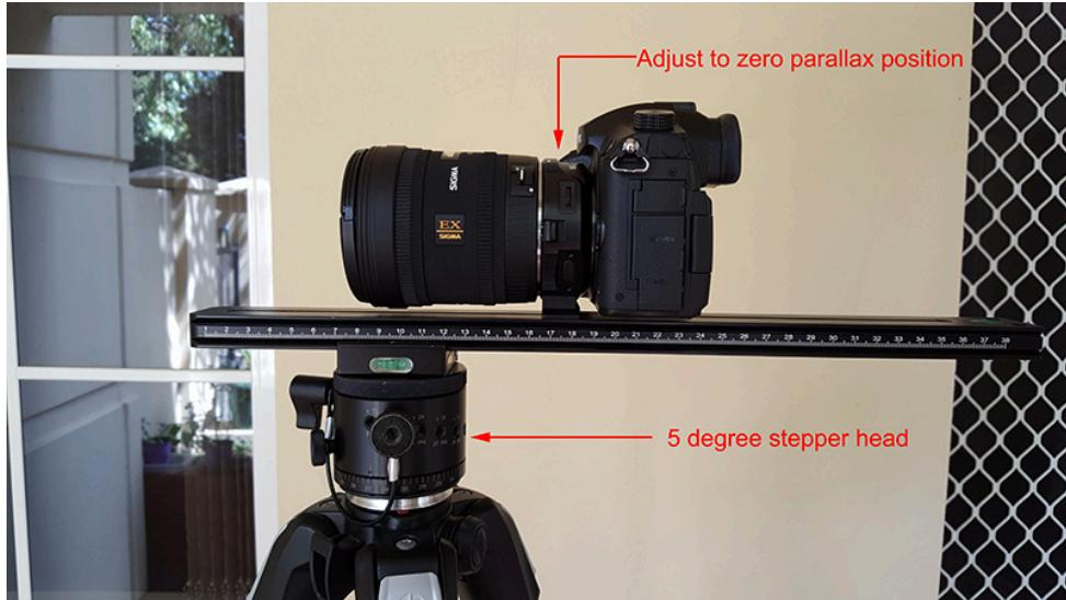
You choose a marker in the scene (eg: line on a wall) and rotate the camera/lens in equal angle steps and take a photograph. Later one measures the position of the marker on each photograph giving "r". Typically one first aligns the camera so the marker line is exactly center of the frame. One also typically rotates from  $-\theta_{\max}/2$  to  $\theta_{\max}/2$ , for example
