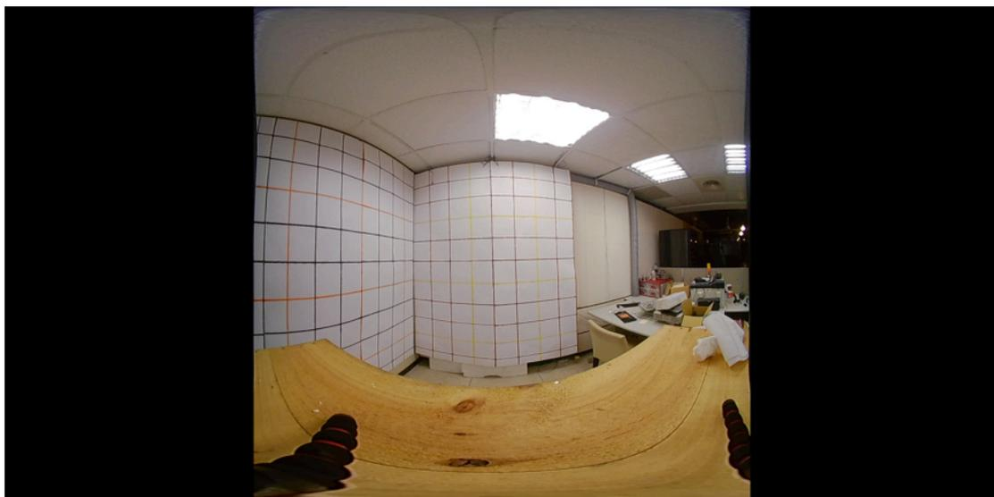
In order to get the best result the various real life optical and geometric properties of the system need to be determined and corrected. In the above it is observed that on the left of the image the lines on the wall are curved, this is an indication that the fisheye field of view is incorrect. Bowed as shown means the angle is too small, bowed the other way means it is too large.
