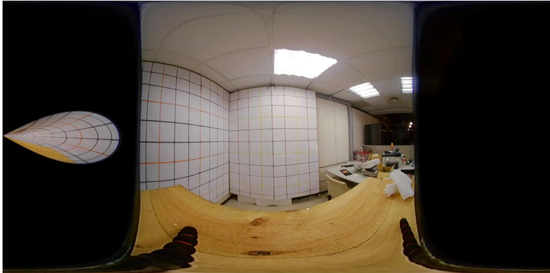
Note: the strange shape in the left black area of the image is the projection of the left hand fisheye image as if the whole input image were a fisheye. Since the purpose here is to create a whole spherical from two fisheyes each fisheye needs to contribute 180 degrees field of view. One can turn on blending but for now with a tiny blend zone to crop to  $\pm 90$  degrees.
