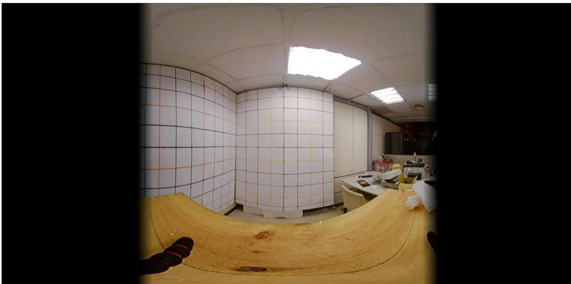
The edge blending assumes a linear combination with the edge blend from the other converted fisheye. After applying the same process to the other fisheye, left and right half of the other converted spherical projection should be positioned on the right and left of the above image. Due to the construction the left and right edges of the resulting spherical image will form a perfect match.
