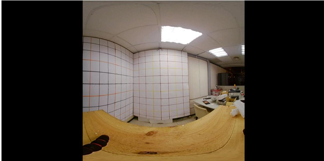
The center vertical line is not straight, this indicates the fisheye lens is not vertical. The axis along the fisheye lens is the y axis, so a rotation through that axis can be applied.
