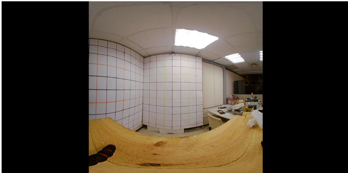
The wall lines on the left are not vertical, this generally indicates the fisheye lens is tilted downwards. The x axis is to the right so a correction can be applied by rotating about that axis.
