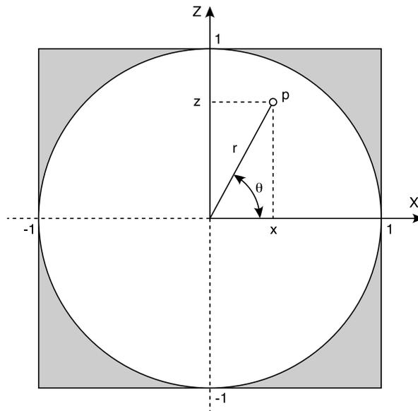
Any 2D point p on a this fisheye image can be parameterised in polar coordinates (r,θ). These r, ϕ, θ are given by
