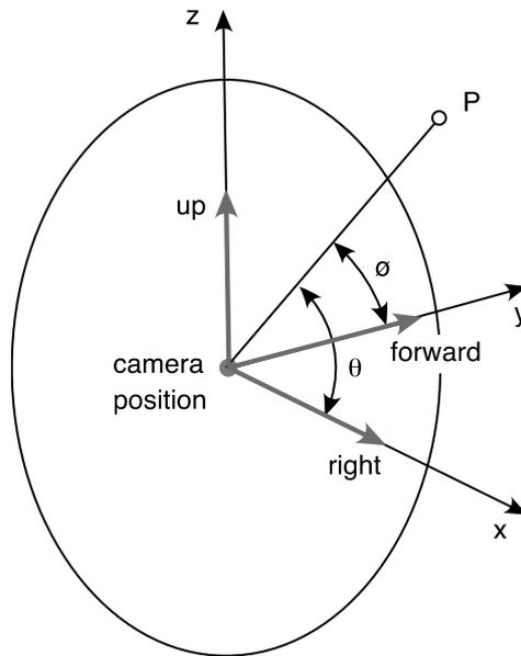
When mapping a fisheye image into an equirectangular projection one needs to calculate the longitude and latitude defined, conventions used here are as below
