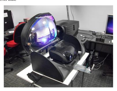
As a historical note the first known record the author is aware of where a spherical mirror used for dome projection dates back to 1957. In this case, before computer graphics, the film was created using a geometrically identical arrangement for filming as for projection (film camera pointing at a spherical mirror). Such techniques where footage is captured by filming with a video camera and a spherical mirror don't apply to computer generated content.
