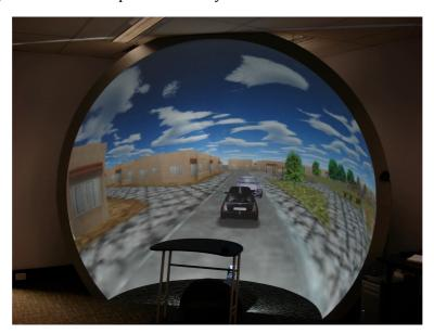
For small domes the main benefit of the spherical mirror approach is that the projection hardware is located well away from the centre of the dome.
