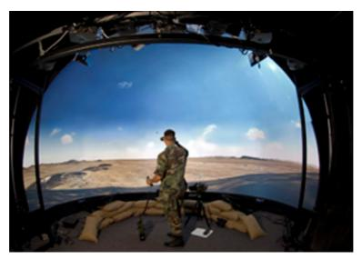
Twin projectors using a pair of spherical mirrors, as far as the author is aware, has not been attempted. The edge blending between the two images is likely to be very challenging.
