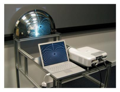
The non-equal size of pixels on the dome is important when designing where the projector and mirror should be placed for any particular application and dome orientation. For the traditional iDome of the author the highest resolution pixels are towards the lower and center of the iDome, the largest pixels towards the top of the iDome. This is an appropriate match to most content, ie: one does need high resolution to represent the sky.
